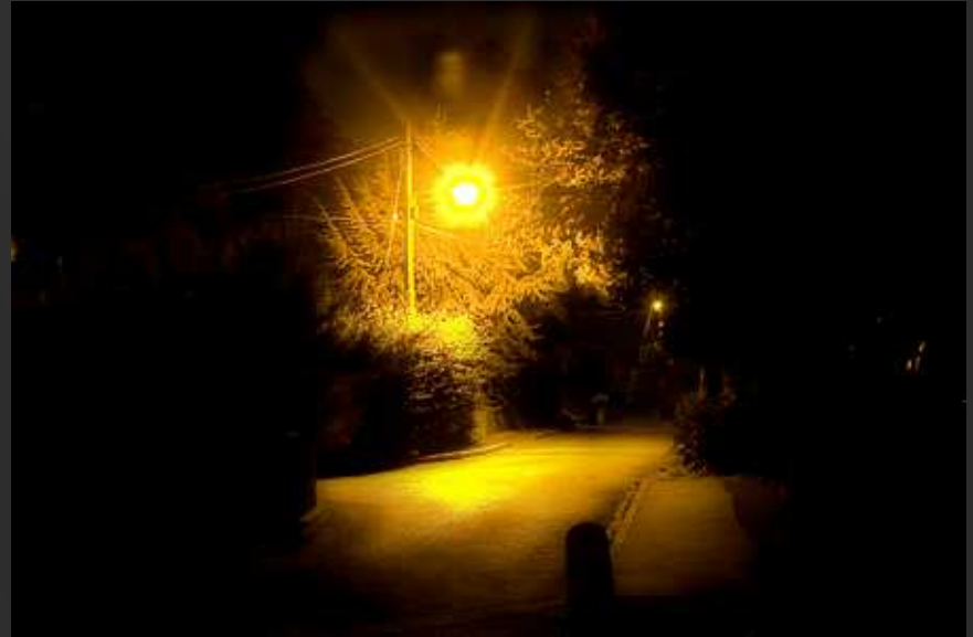
Old style, very prevalent, exposed luminaire, blinds onlooker, causes light pollution, wastes energy
