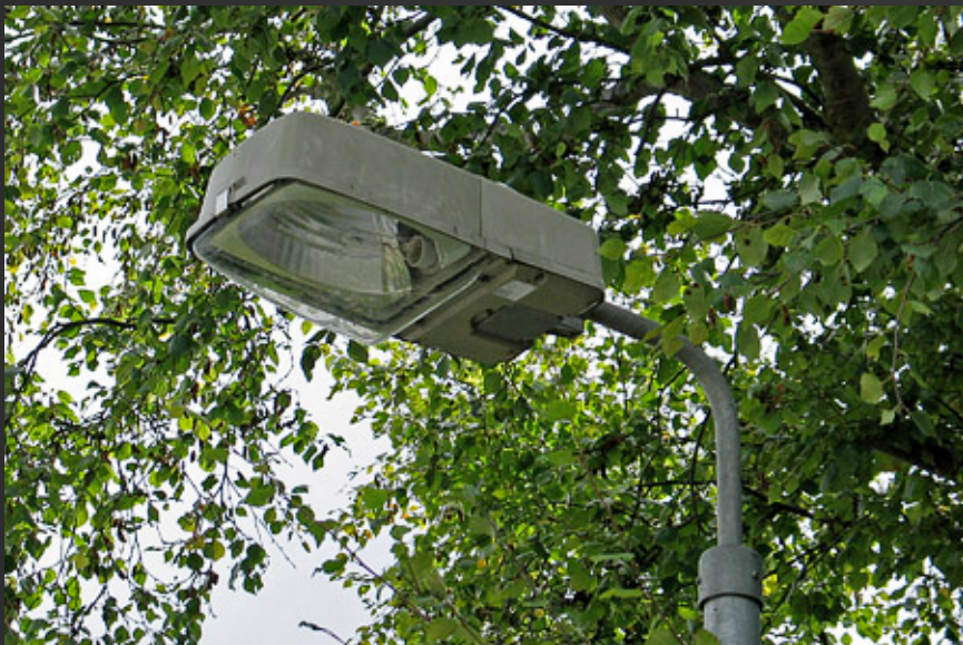
Newer style, less prevalent, partially shielded luminaire, less light pollution, less energy waste, much better illumination
